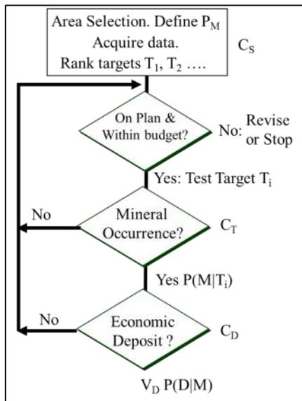
**Figure 1. Simplified flow chart of an exploration program.**
